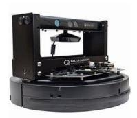
The Quanser QBot 2e is an innovative open-architecture autonomous ground robot, equipped with built-in sensors, and a vision system. Accompanied by extensive courseware, the QBot 2e is ideally suited for teaching undergraduate and advanced robotics and mechatronics courses, surpassing capabilities of hobby-level robotic platforms.
