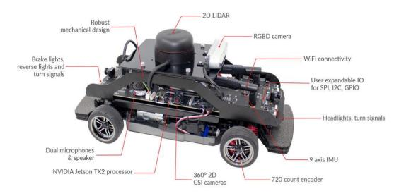
At the center of the Self-Driving Car Research Studio, the QCar, is an open-architecture scaled model vehicle, powered with NVIDIA® Jetson $^{\text{TM}}$  TX2 supercomputer, and equipped with a wide range of sensors, cameras, encoders, and user-expandable IO.
