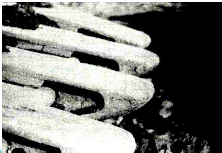
4-rasm. Ekskavator cho'mich tishining yeyilish natijasida shaklining o'zgarishi
