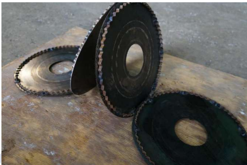
3-rasm. Arraga qistirmalarni payvandlash.
